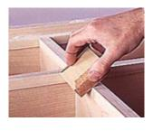
11--Put a small, crisp bevel on the facing and edge strips with a sanding block that you move perpendicular to the strip's edge.
