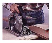
1--Clamp a straightedge across the workpiece and crosscut it with a circular saw. Support the piece that will be cut off.
