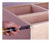
8--Use a chisel to cut a small clearance notch in the top corner of each vertical facing strip. Cut in toward the case.
