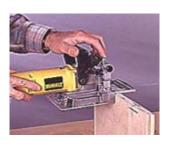
4--Clamp the case sides upright in a vise and cut the slots along their upper edge using the plate joiner's fence for alignment.
