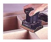
10--Sand the surfaces carefully using a randomorbit block sander. This tool is small enough to fit into the compartments.
